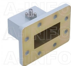
187WCAS Right Angle Rectangular Waveguide to Coaxial Adapter 3.95-5.85GHz WR187 to SMA Female
